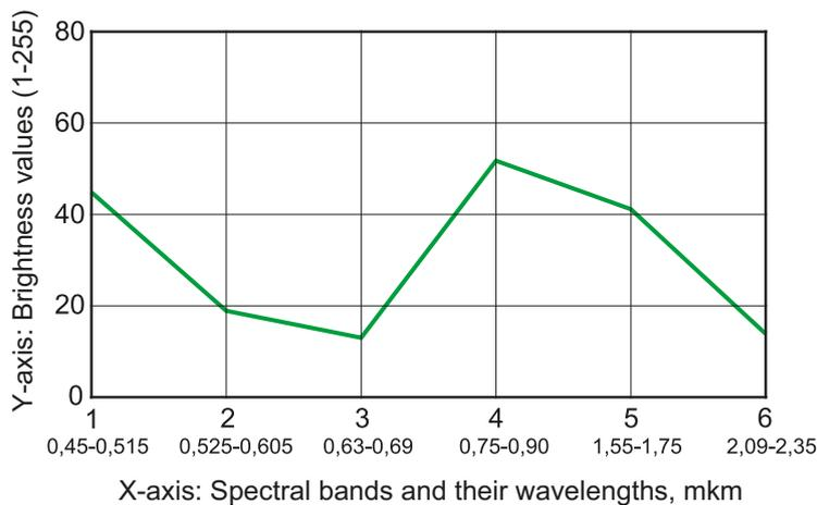
Fig. 2.21. Spectral characteristics of spruce and aspen in the channels of the Landsat TM/ETM+ images.
