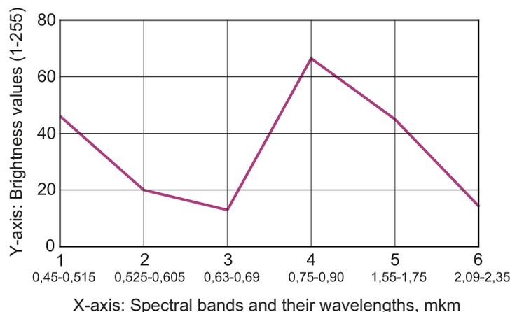
Fig. 2.22. Spectral characteristics of secondary forest dominated by birch and aspen in the channels of the Landsat TM/ETM+ images.
