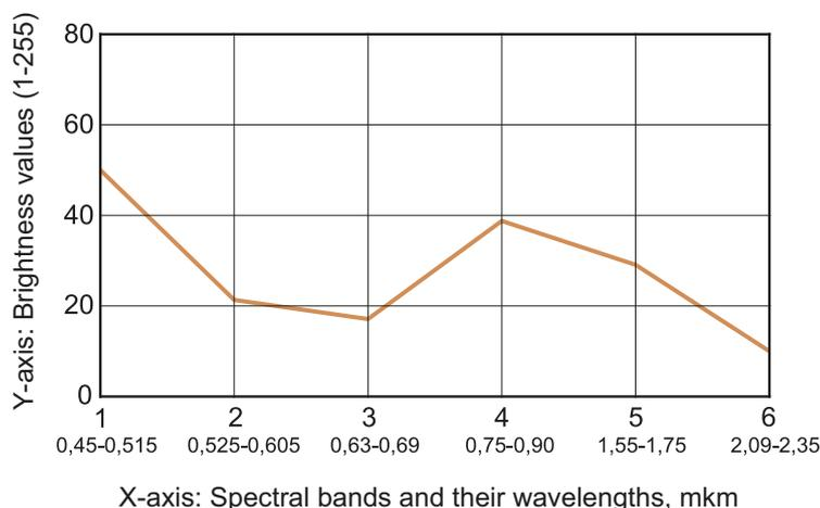
Fig. 2.27. Spectral characteristics of forests including significant amount of larch from satellite images Landsat TM / ETM +.
