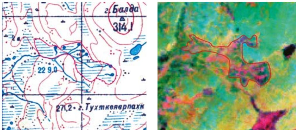
Fig. 2.19. Selection of spring fens: how the spring fen was represented in the topographic map (left) and how it is analyzed in a Landsat TM satellite image (right).
